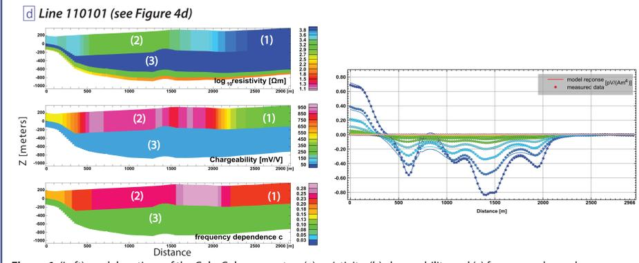
(1) high-resistivity eastern part (4 000 Ohm.m): correspond to outcropping basement - low chargeability (300 mV/V)
