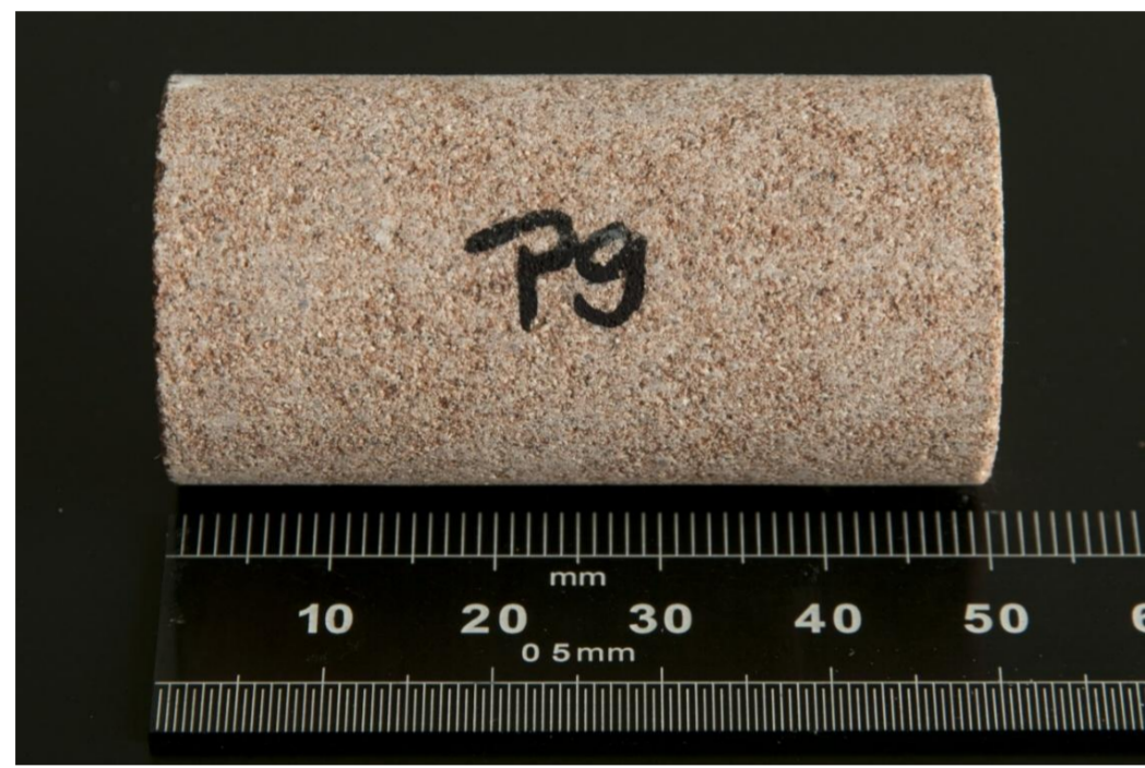
Fig. 5: Sandstone sample P9, used for the SIP measurements at varying temperature and salinity.
