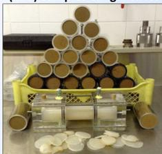
**Box III: Installation.** The sample holder and the samples are stored in a climate controlled chamber set at 20°C and 50% humidity (A). We conducted preliminary tests with the sample holder filled with agar gel to ensure the measured residual phase is below 1 mrad. The agar gel was renewed between the measurements on group N and group T.
