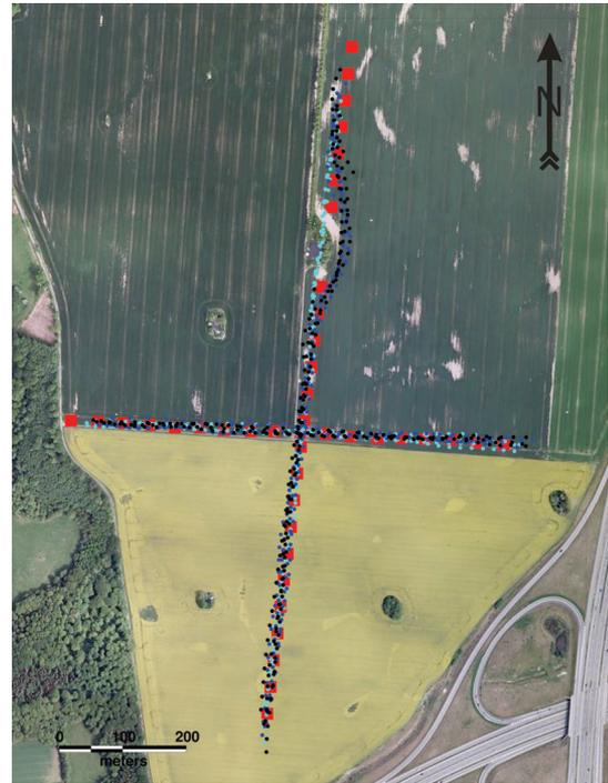
Figure 2. Detailed map of the Danish TEM test site. Red squares mark the two reference lines (ground-based TEM soundings). The point reference site is at the line intersection. Black, blue, and cyan dots mark the different SkyTEM repetitions from the validation data set.
