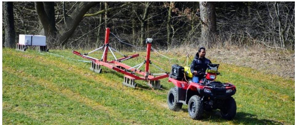
Figure 1. The tTEM system in action.
