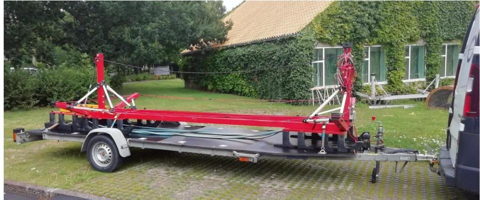
*Figure 4. The tTEM system packed on the transport trailer. The ATV and all instrumentation is inside the van.*
