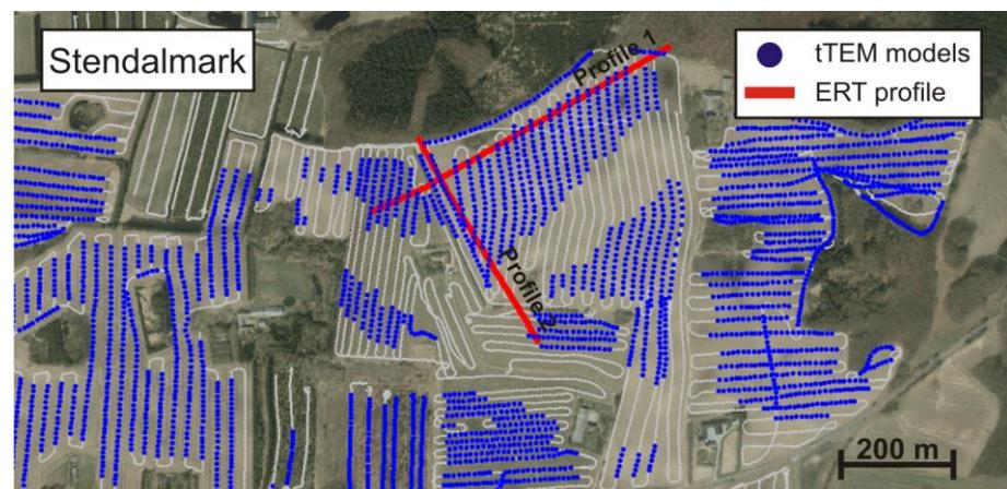
Figure 36. Part of Stendal Mark tTEM survey. Gray dots are the tTEM survey lines, overlain with the blue dots marking coupling free data invited to resistivity models. Red lines mark the two ERT profiles.
