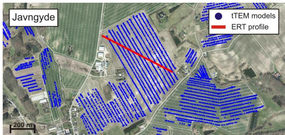
Figure 39. Part of tTEM survey in Javngyde (blue dots) and location the ERT profile.
