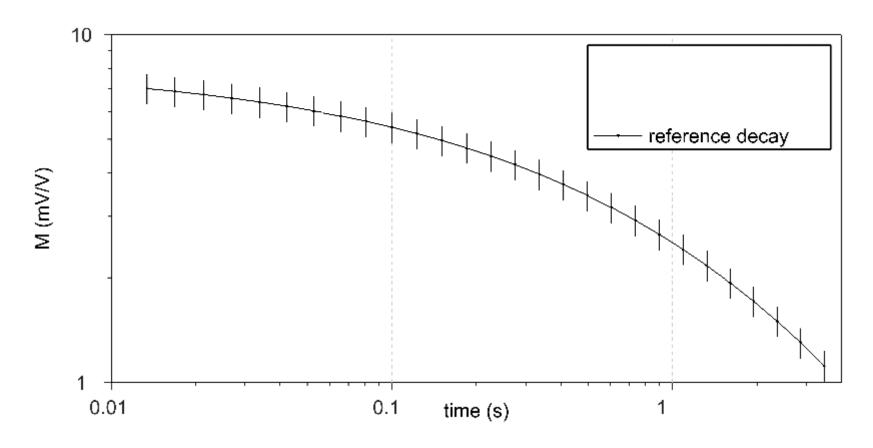
Forward response for homogeneous halfspace ( $\rho$ =100  $\Omega$ m,  $m_o$ =10 mV/V,  $\tau$ =1 s, C=0.5)
