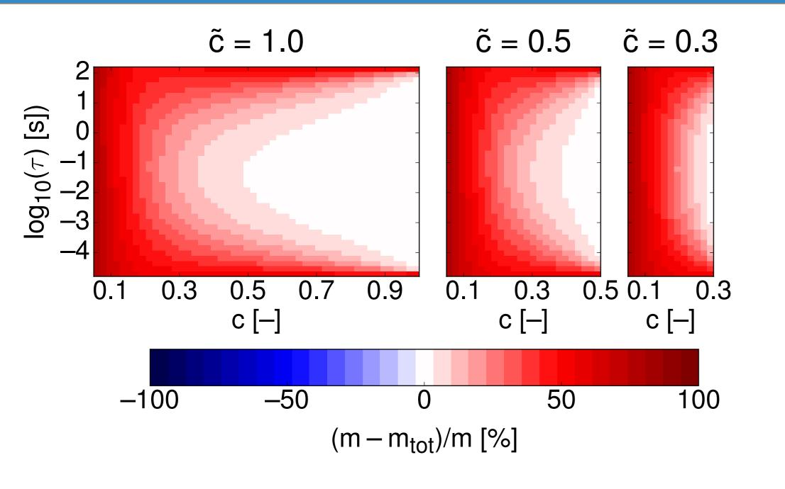
The total chargeability  $m_{tot}$  increasingly underestimates the original CC based m parameter with decreasing cvalue and with  $\tau$  approaching the relaxation time limits. This behavior is observed for different CC kernels and is compressed within the range  $c \leq \tilde{c}$ .
